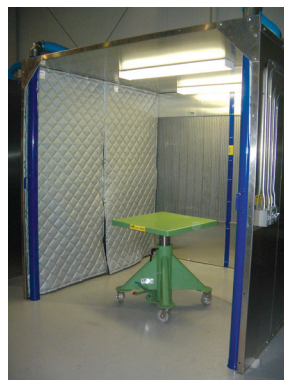
W18/8 8' Walk-In Clean Air Station
