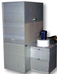
Rear View with Smoke/Fume Collection Filter Housing
